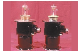
2 MW S-band magnetrons for DAE
