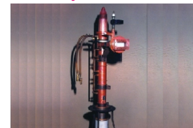
5 MW S-band klystron for DAE
