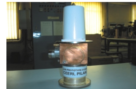
2.6 MW S-band magnetron for SAMEER
