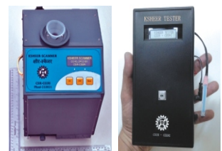
Ksheer scanner/tester for detec- tion of adulteration in milk
