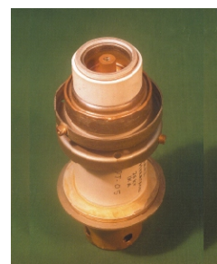
25 kW/1 kA hydrogen thyatron
